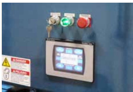
The touchscreen allows full automatic and manual control with one touch. Screens may be customized, password protected, and are designed with alarm, diagnostic and help screens.
